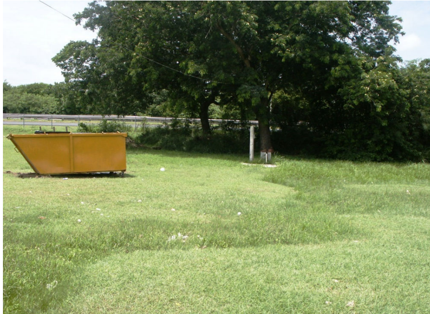
Figure IV.C.5. Well with possible surface sources of contamination; note ditch from cistern/wastewater overflow and dumpster.
