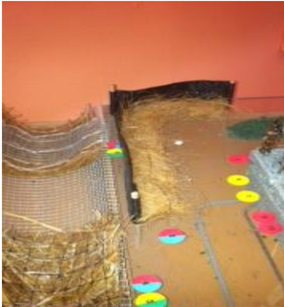
Fig. 5 Model house depicting the use of a silt fence and brush berm as a best management practice (BMP's)
