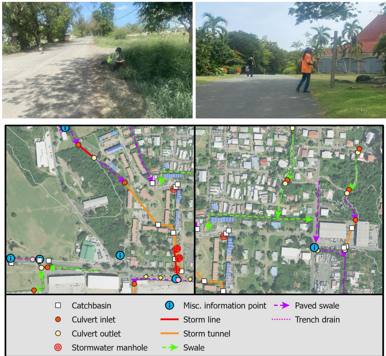
Figure 49. Inspection of existing stormwater infrastructure during field assessments (above) and an
