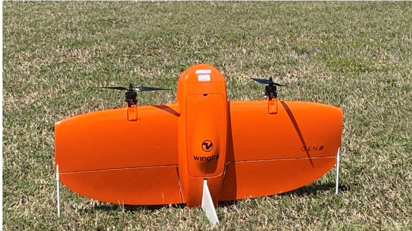
Figure 50. WingtraOne Gen II UAS utilized to collect data in the study watersheds.
