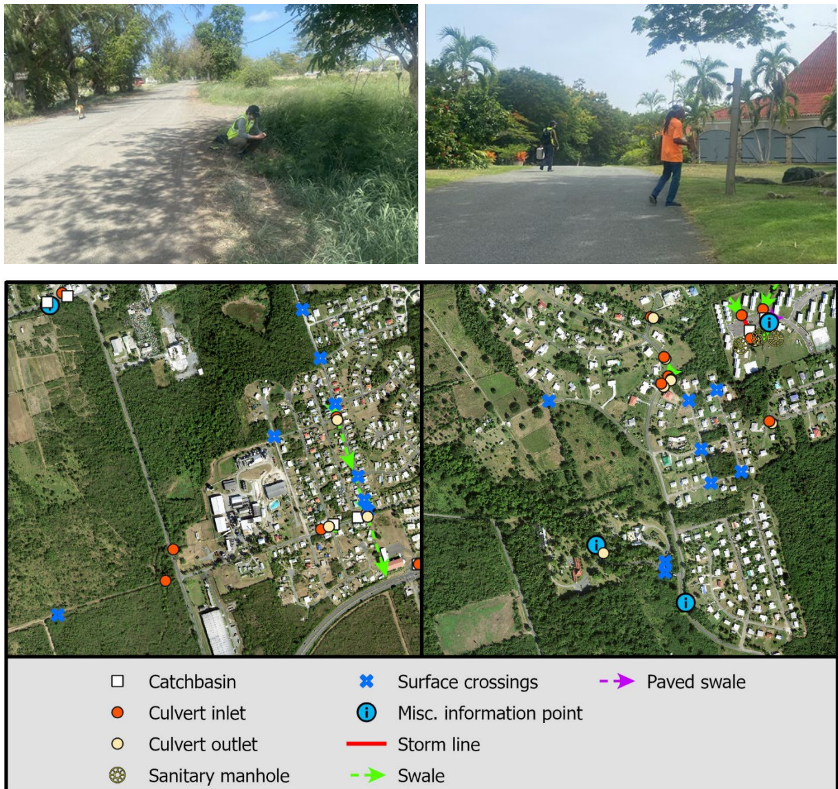
Figure 46. Inspection of existing stormwater infrastructure during field assessments (above) and an example of the maps produced (below).
