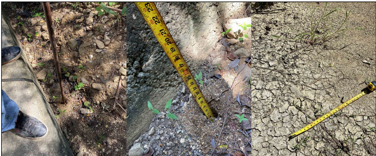
Figure 54. A sediment core being collected from the Dia02 gut channel (left). The depth of the sediment core verified with measuring tape (center). A cross-section across the Dia02 gut channel measured to collect a scrape sample (right).
