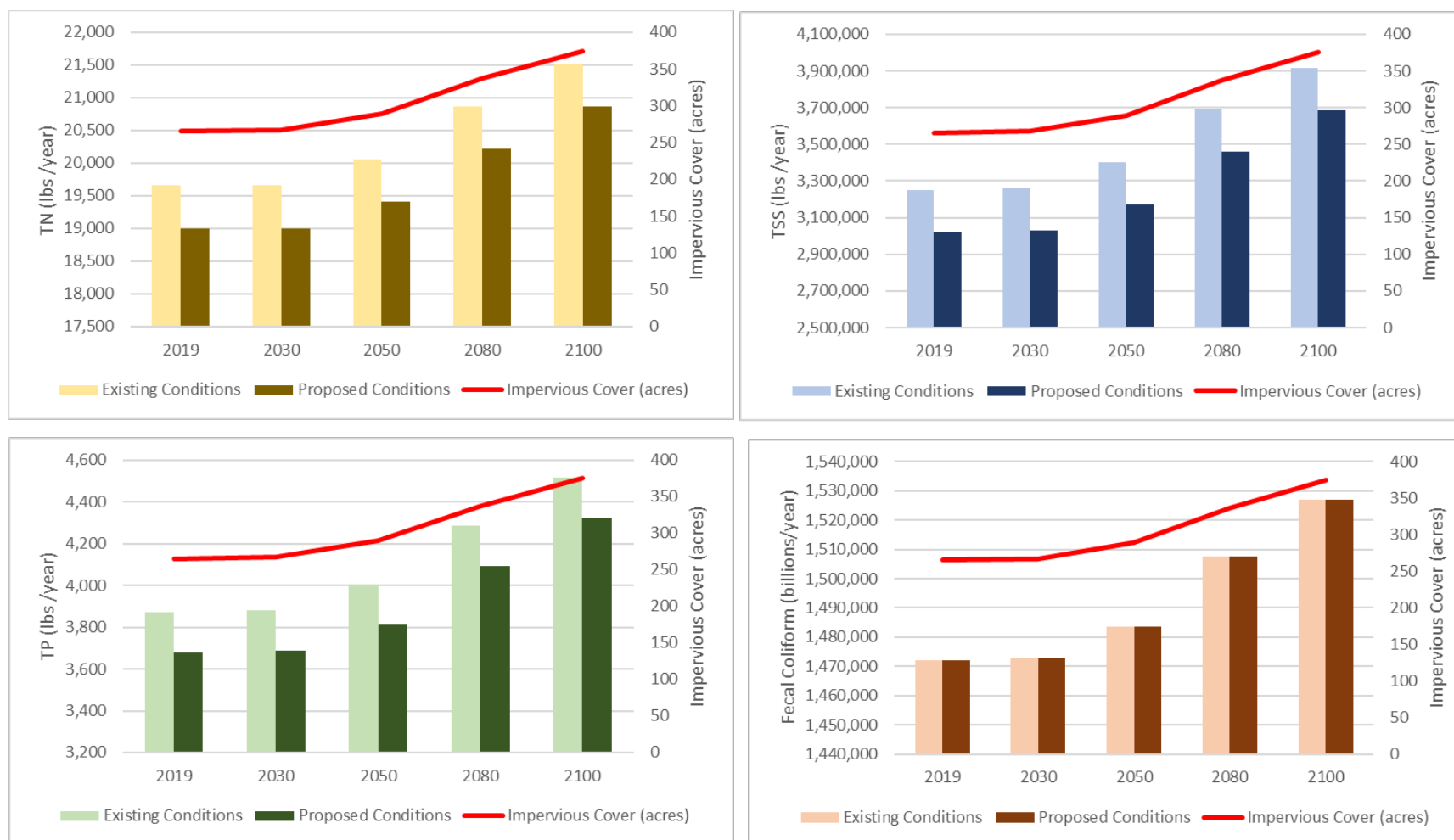
Figure 83. Relationship over time between watershed scale pollutant loading for the existing conditions (lighter colors) and proposed conditions (darker colors), which includes the implementation of the Top 10 BMPs. Loading is shown for TN (yellow), TSS (blue), TP (green), and Fecal Coliform (orange). The predicted impervious cover increase (red line) over time is also shown.
