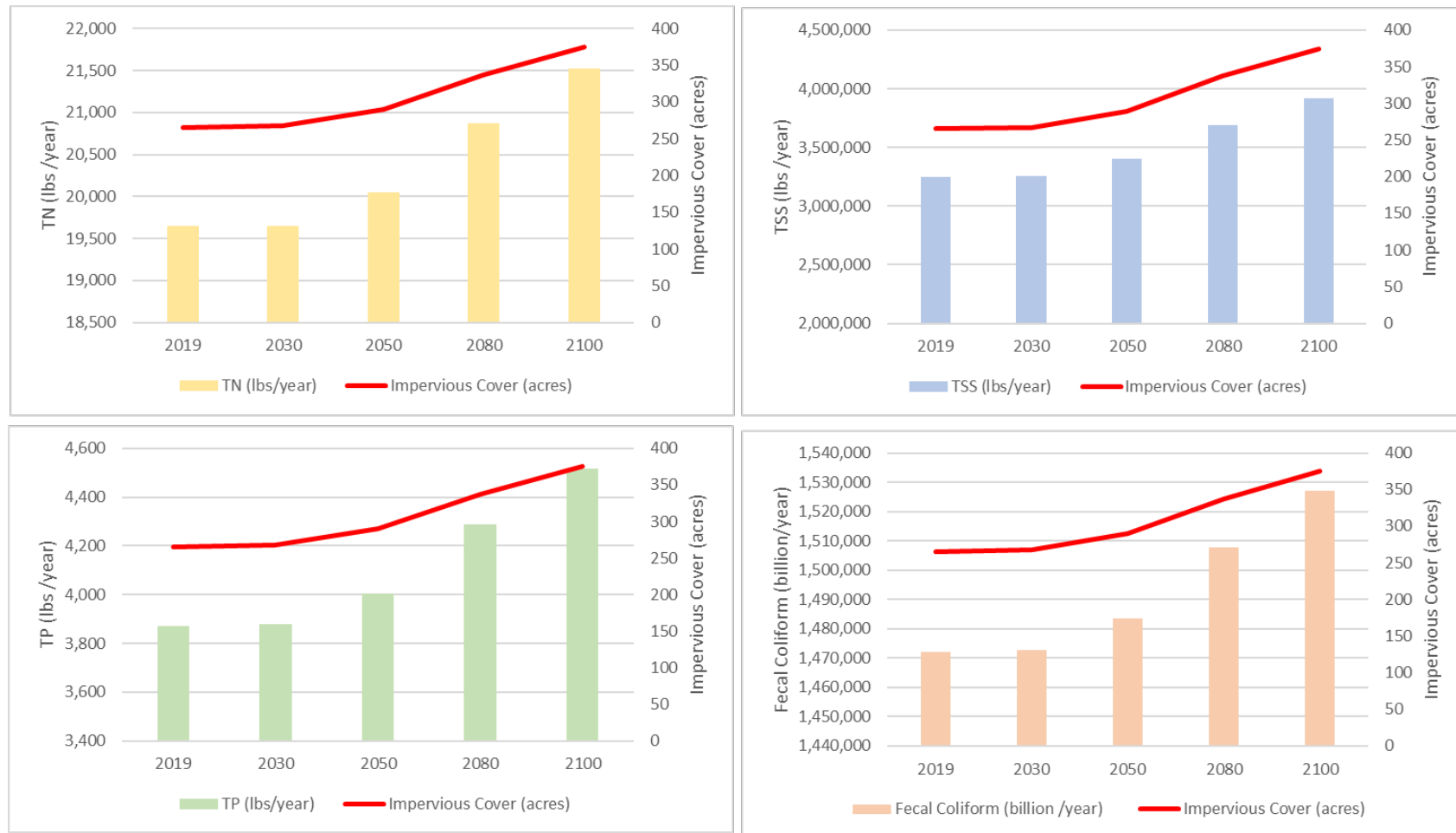
Figure 78. Relationship between watershed-scale pollutant loading for TN (yellow), TSS (blue), TP (green), and Fecal Coliform (orange) and the predicted impervious cover increase (red) over time.
