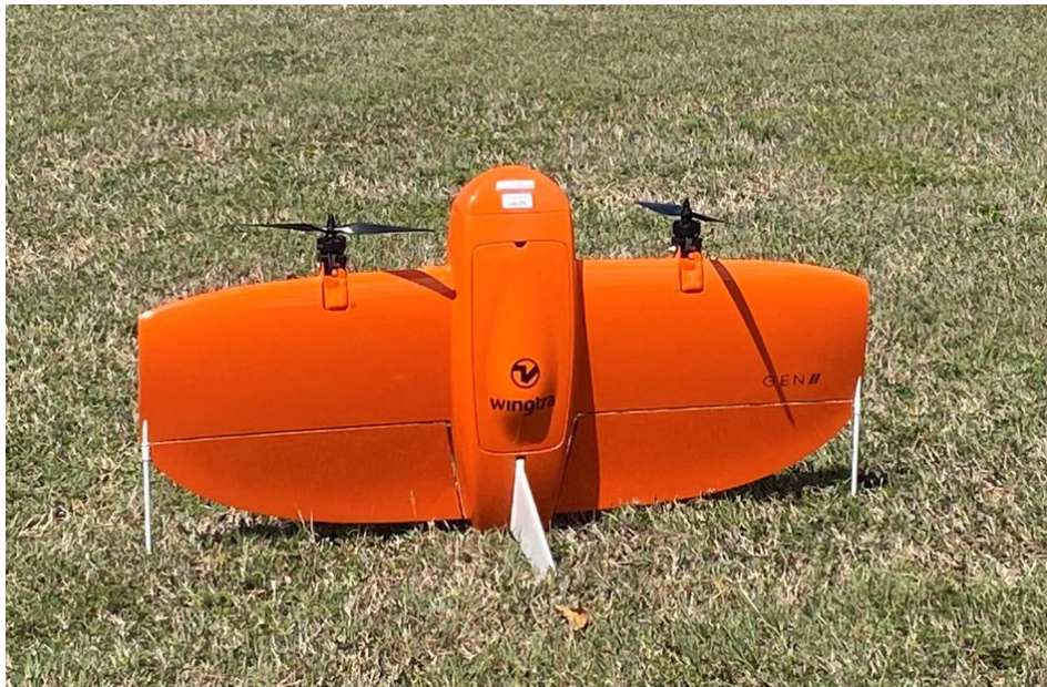
Figure 48. WingtraOne Gen II UAS utilized to collect data in the study watersheds.
