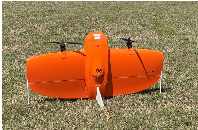
Figure 55. WingtraOne Gen II UAS utilized to collect data in the study watersheds.
