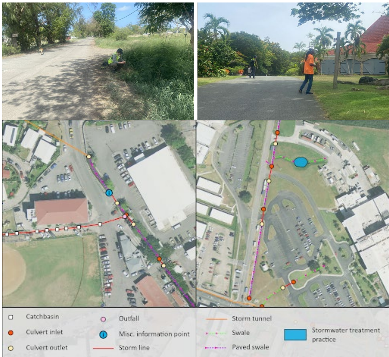
Figure 52. Inspection of existing stormwater infrastructure during field assessments (above) and an
