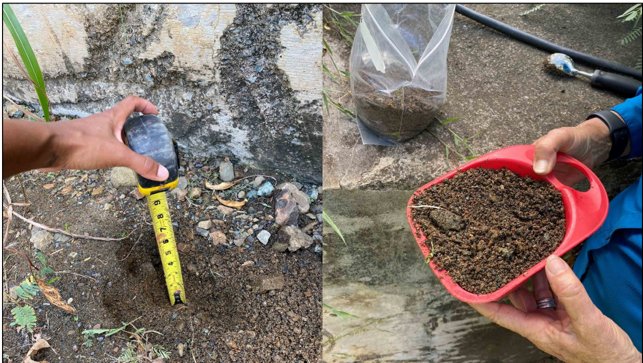
Figure 61. Field crew member measuring the depth of deposition (left) and collecting a subsample of the various sediment types across the cross-section of the gut channel (right).
