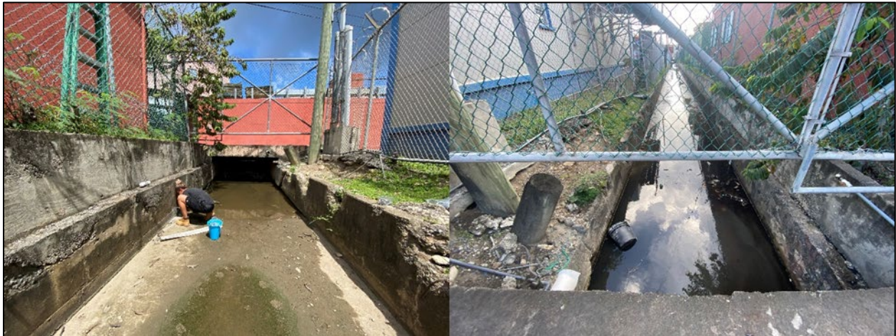
Figure 60. Field crew member setting up an Onset HOB0 U20 Water Level Logger at gauge station (left) and water flowing through the gut following a rain event (right) at STH 01.
