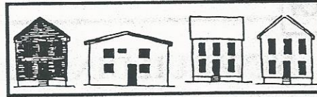
Elements such as the size and placement of windows, the height of the first floor above grade, the roof shape and pitch, and the building's orientation are probably the most important factors to consider when designing new buildings.
