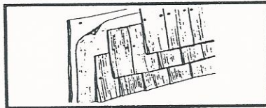
Cedar shingles - a common siding material for wood buildings in the Virgin Islands.
