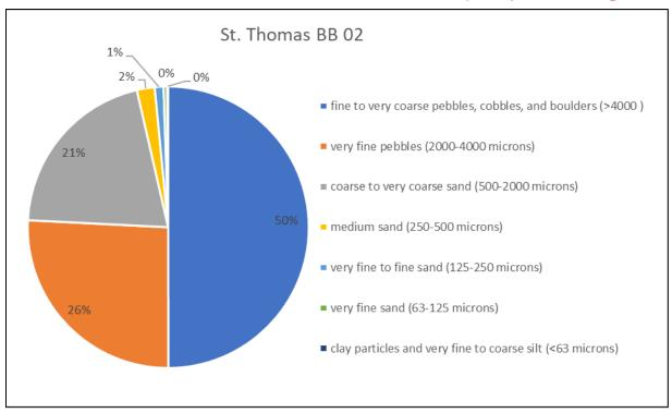
Figure 62. The percent composition of the seven grain size categories within the BB02 sediment sample.
