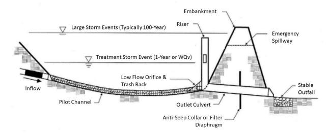
Figure 73. Dry detention basin design. Graphic adapted from the 2017 Vermont Stormwater Management Manual Rule and Design Guidance (Vermont ANR, 2017).
