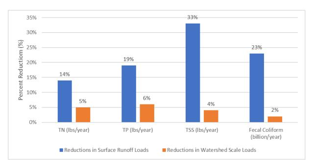
Figure 74. Pollutant load reductions attributable to the Top 10 BMPs for the Surface Runoff category (blue) and for all modeled watershed sources (orange).
