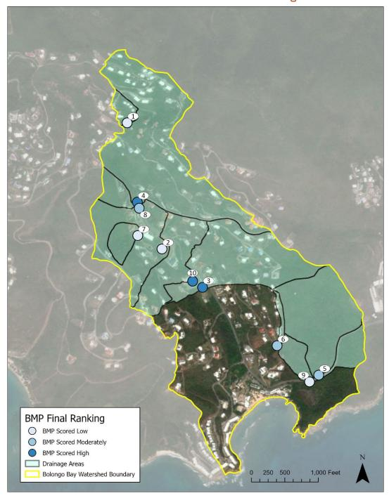
Figure 67. The relative ranking of each BMP and the associated BMP drainage areas. Note that drainage areas for BMPs often overlap.
