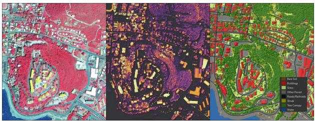
Figure 29. Imagery displayed as color infrared (left), LiDAR nDSM (center), and resulting land cover (right) on an example area in St. Thomas Island.
