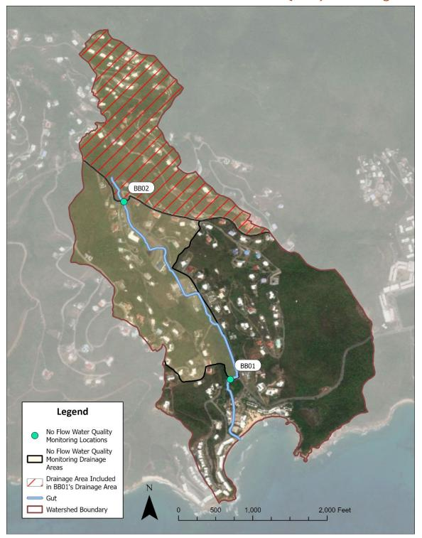
Figure 59. The BB01 and BB02 monitoring locations were confirmed to have no storm flow during five qualifying rain events between October and December of 2021. The BB01 drainage area is delineated in light yellow and the BB02 drainage area is shown with red diagonal lines.
