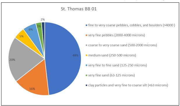
Figure 61. The percent composition of the seven grain size categories within the BB01 sediment sample.
