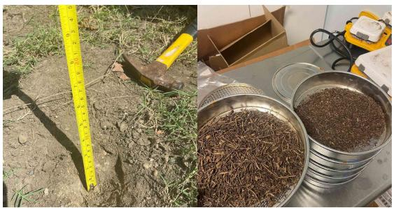
Figure 55. Field crew member measuring the depth of deposition (left) and separating a subsample of the various sediment types across the cross-section of the gut channel (right).
