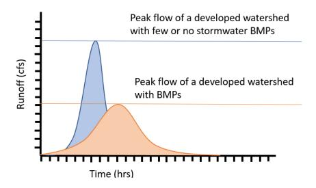
Figure 72. Illustrative hydrographs demonstrating the peak flow reduction value of implementing BMPs.
