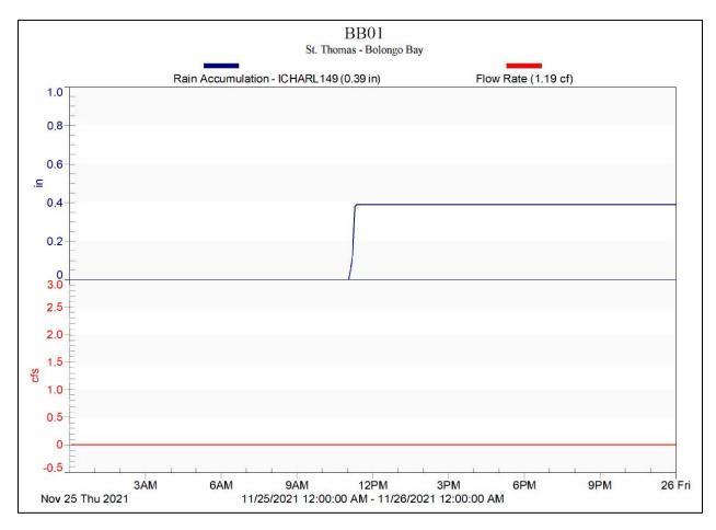
Figure 57. A hydrograph displaying the lack of flow at the BB01 gut monitoring site (0.0 cfs) in red and the corresponding rain accumulation for the storm event (0.39 in.) in blue that occurred on November 25th, 2021.
