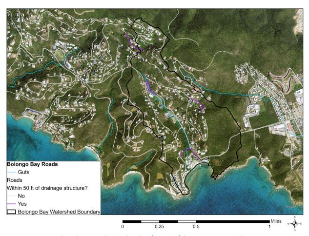
Figure 37. Roads in the watershed and a classification of distance to nearest drainage structure.
