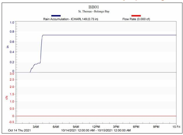
Figure 56. A hydrograph displaying the lack of flow at the BB01 gut monitoring site (0.0 cfs) in red and the corresponding rain accumulation for the storm event (0.73 in.) in blue that occurred on October 14th, 2021.
