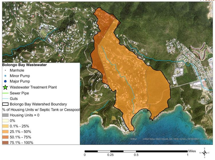
Figure 38. Sanitary sewer system and percent of housing units by estate with septic tanks or cesspools in the Bolongo Bay watershed (Sources: 2010 U.S. Census data, VIWMA).
