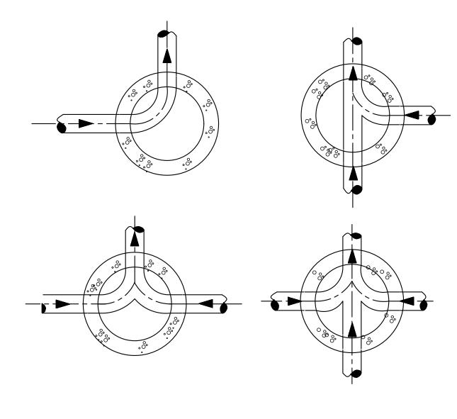
INVERT CHANNEL FLOW DIRECTION Detail N.T.S.
