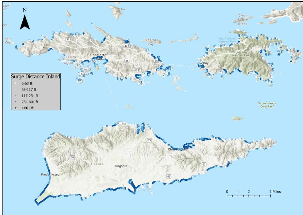
Figure 16: Storm surge inundation distance from the coast as computed by the SLOSH model<sup>9</sup>
