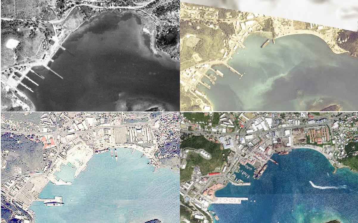
Figure 25: Expansion of the port infrastructure in St. Thomas from 1954 (top left), 1970 (top right), 1980 (bottom left), to 2020 (bottom right).
