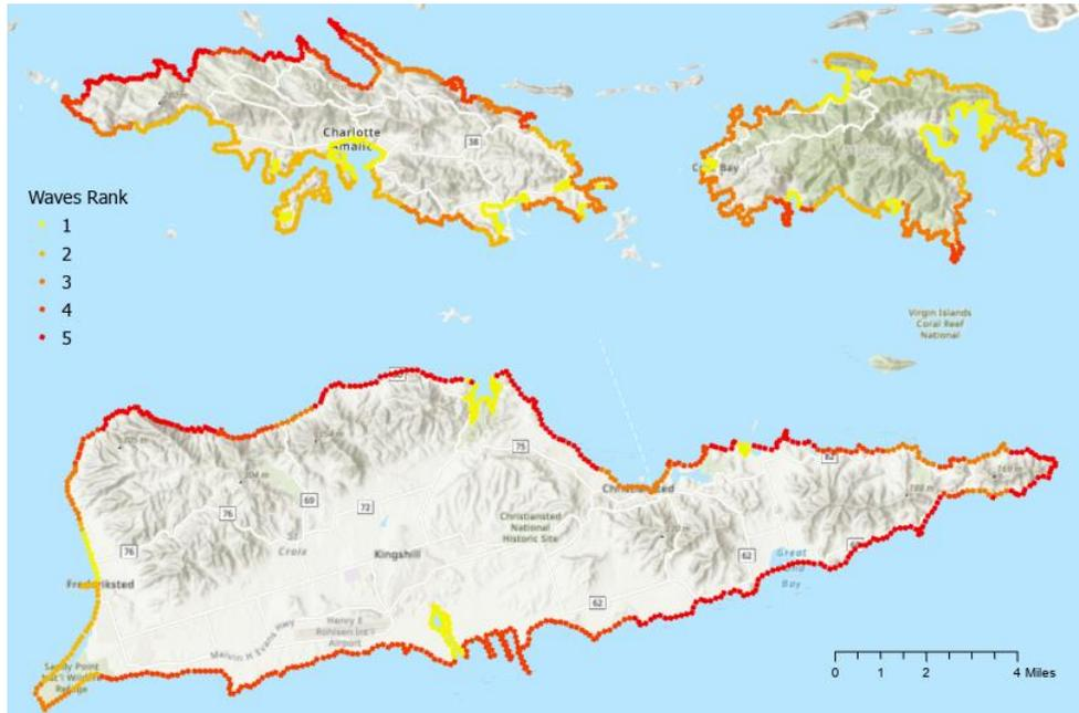
Figure 20: Wave power ranking for the USVI.
