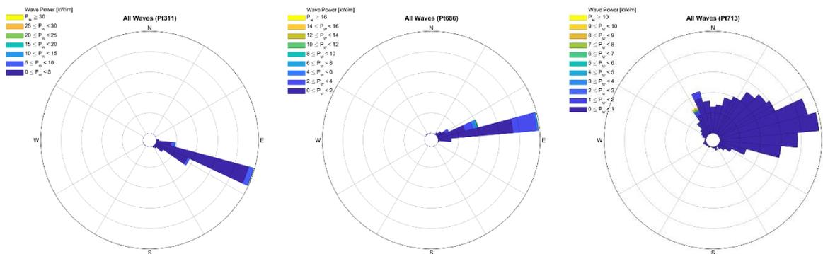
Figure B8: Wave rose for discrete points around St. Croix: Northeast (Pt. 311), Southeast (Pt. 686), and Northeast (Pt. 713)
