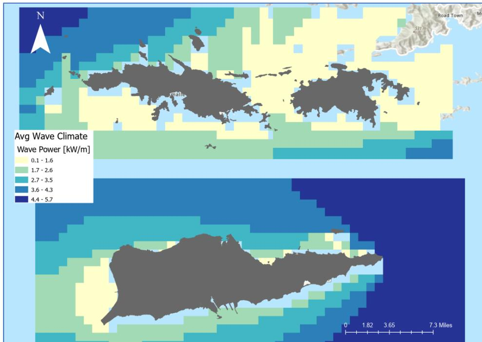
Figure 18: Wave power climate around the USVI
