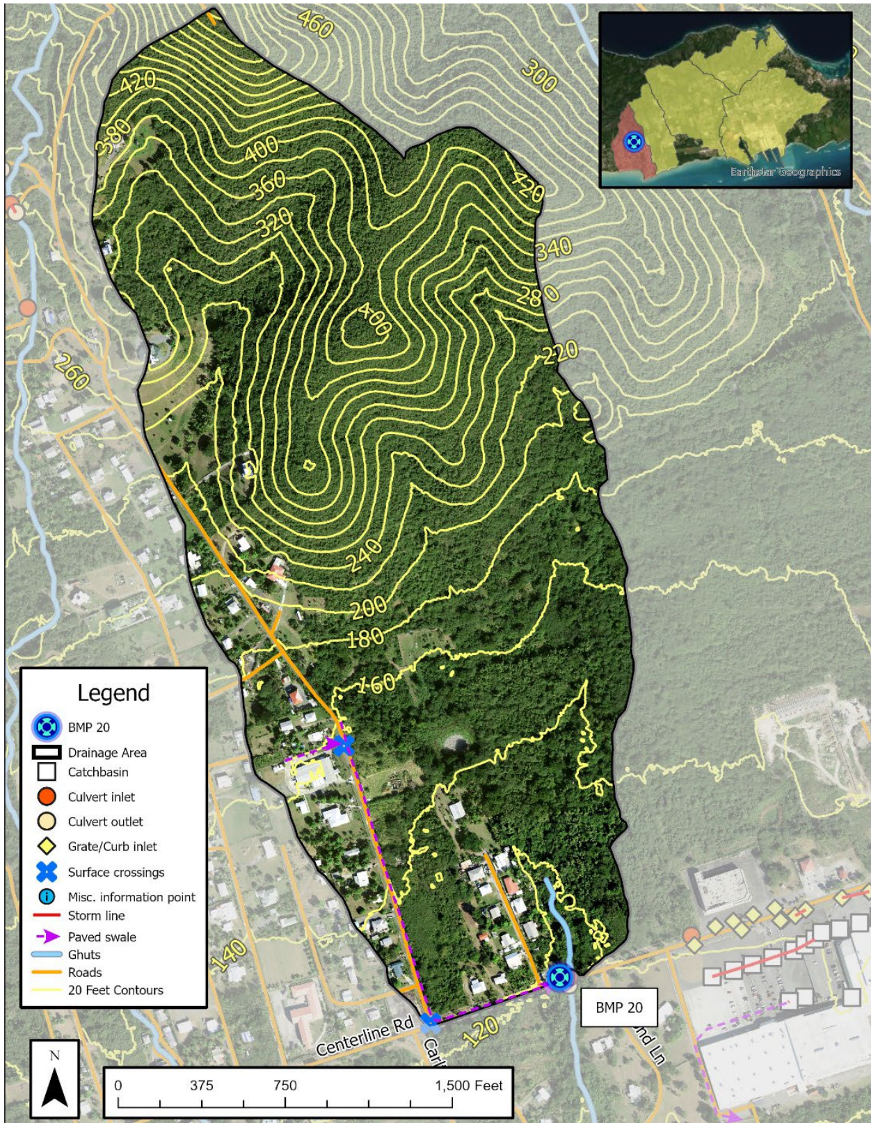
Figure 80. BMP 20's drainage area and its associated infrastructure
