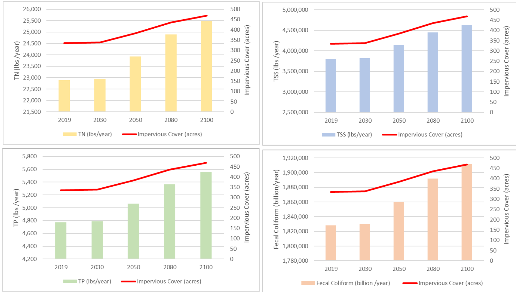
Figure 83. Relationship between watershed-scale pollutant loading for TN (yellow), TSS (blue), TP (green), and Fecal Coliform (orange) and the predicted impervious cover increase (red) over time.
