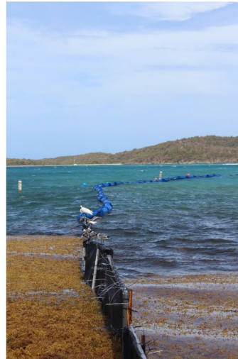
Figure 6.0 Boom channeling sargassum influx to the left side of the bay for mechanical collection at the Ritz-Carlton, St. Thomas.
