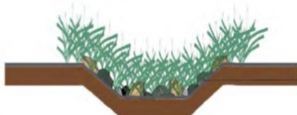
Figure 4.22. Combination vetiver and stone check dams in Culebra, PR. Vetiver check dam detail with armoring options for higher flow channels (from CBCC, 2017). The vetiver grass helps dissipate energy, trap sediment, and soak up standing water.
