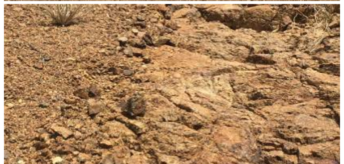
Native soil (top), when loose and unconsolidated is highly prone to erosion. High clay content can make it slippery when wet. Bedrock below a thin layer of sediment (bottom) makes creation of ditches and installation of cross-drains a challenge.
