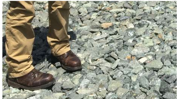
1"-3" stones used as a base course. This stone is also good in ditches and as chocker stone in riprap applications.
