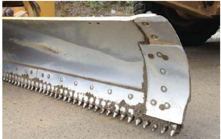
Rotating tipped carbide grader blades are expensive, but worth the investment due to durability, cutting and rock shattering effectiveness, and grooving that improves material compaction and binding.
