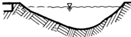
Bucket-shaped, parabolic (preferred)
