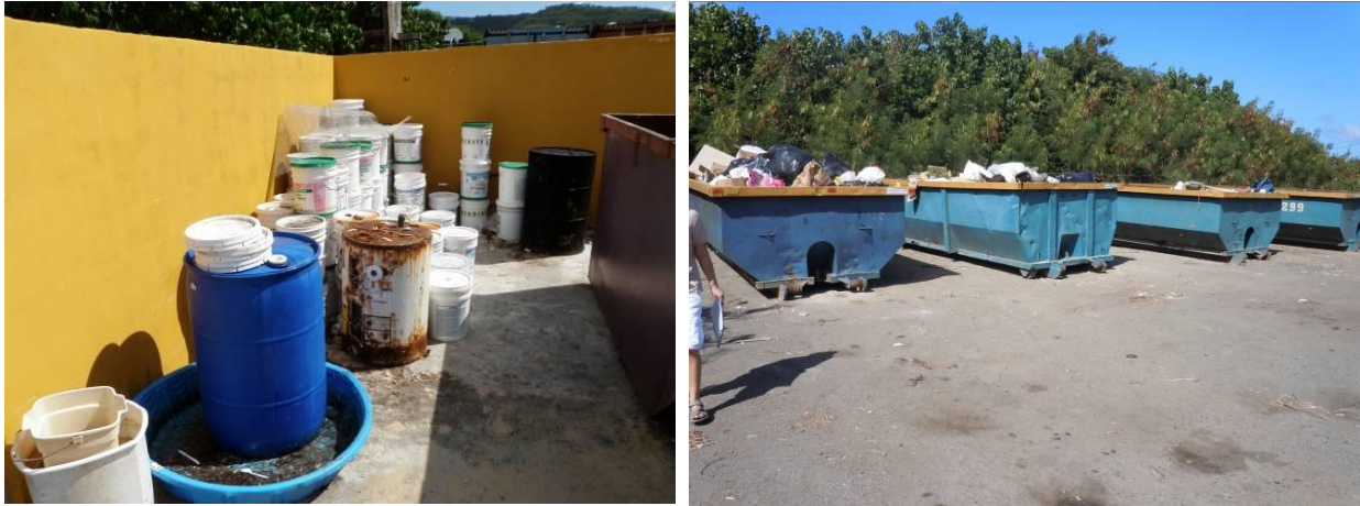
Figure 11. Examples of Outdoor Material Storage and Dumpster Management (note the use of plastic swimming pool as cost-effective secondary containment).
