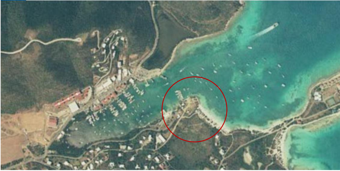
This 1999 shows that one dock was rebuilt, and the remnants of the more easterly dock are present. The easterly dock was destroyed by hurricane Marilyn.
