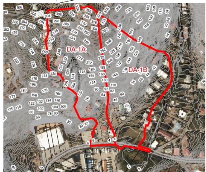
Figure 3.5. The 2,000 SF of impervious cover draining to a rain garden in Hope and Carton Hills, St. Croix (top) and 15-acre drainage area to a restored culvert and trench drain at Independent Boatyard on St. Thomas (bottom).
