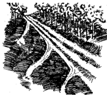
Figure 4.57 Illustrations showing road turnouts from ditches (MA Unpaved Roads BMP Manual) and directly from road surface (Alabama Forest Service).
