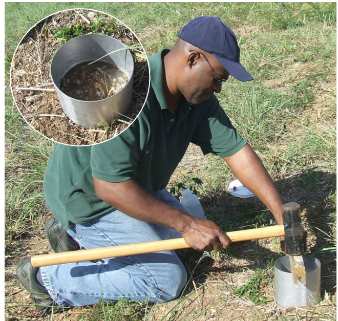
NRCS staff measuring infiltration rates using a single ring infiltrometer at a potential rain garden location on St. Croix.
