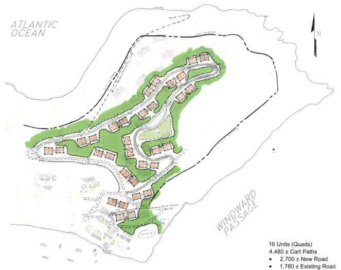
Figure 3.8. Alternative site layout for eco resort on St. John focused on maintaining a 200ft or greater shoreline setback, limited clearing around proposed structures, and a drainage friendly road network.
