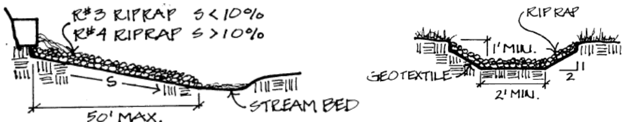
Figure 4.25 Rip-rap channel (source: VT Unpaved Road BMP Manual)
