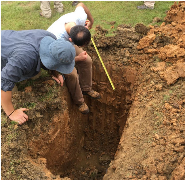
Test pit dug at the Smith Bay ballfield on St. Thomas to measure depth to groundwater and evaluate the soil profile and texture to determine infiltration potential.
