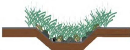
Figure 4.22. Combination vetiver and stone check dams in Culebra, PR. Vetiver check dam detail with armorings for higher flow channels (from CBCC, 2017). The vetiver grass helps dissipate energy, trap sediment, and soak up standing water.
