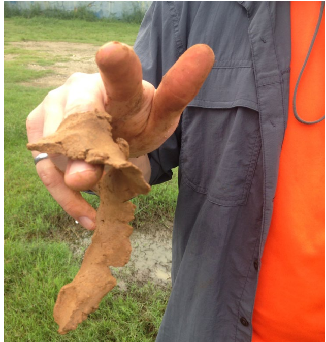
This ribbon test indicates a higher clay content which means that assumed design infiltration rate from Rawls table are less than 0.1 in/hr.
