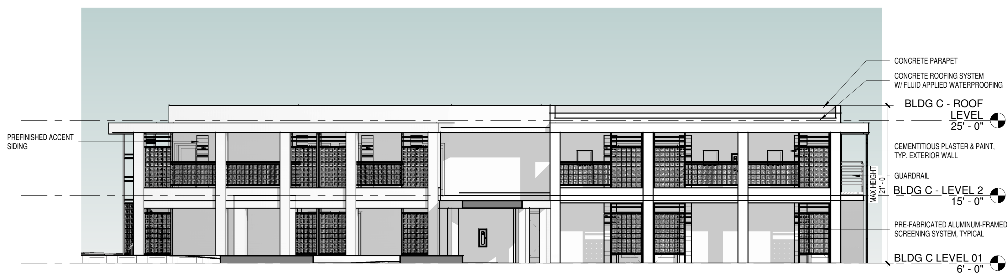
1 BLDG C - SOUTH ELEVATION A-C2.0 SCALE: 1/8" = 1'-0"
