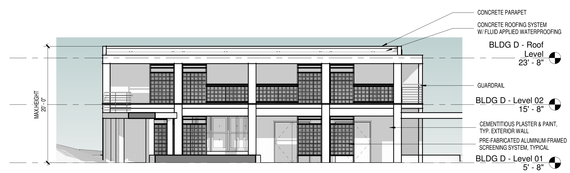
2 BLDG D - SOUTH ELEVATION A-D2.0 SCALE: 1/8" = 1'-0"
