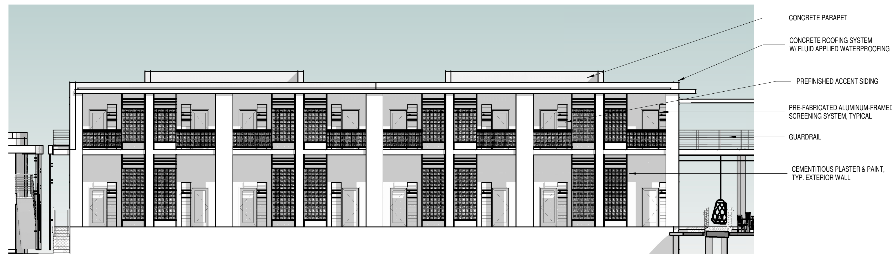
2 BLDG K - WEST ELEVATION A-K2.0 SCALE: 1" = 10'-0"
