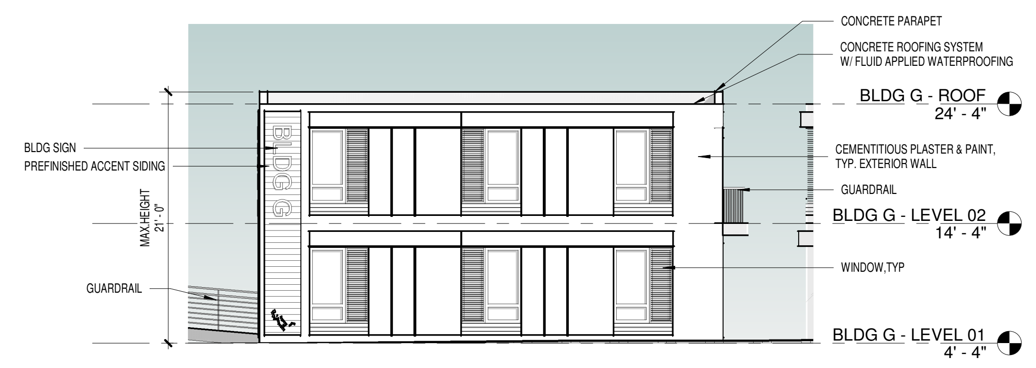
3 BLDG G - NORTH ELEVATION A-G2.0 SCALE: 1/8" = 1'-0"
