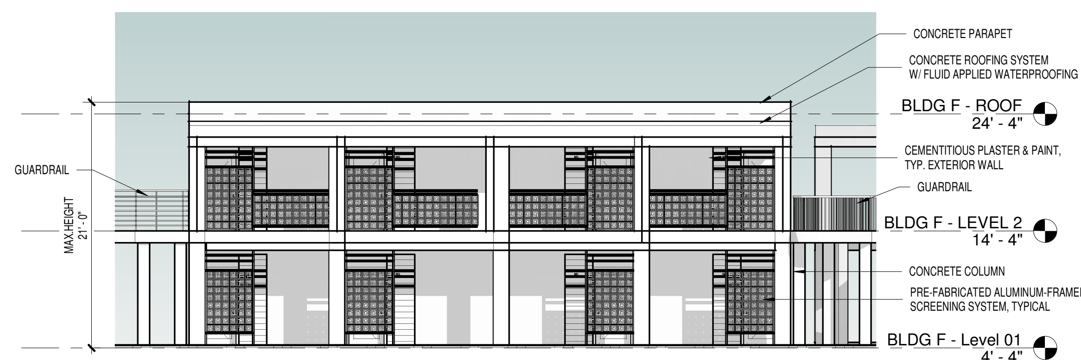
1 BLDG F - SOUTH ELEVATION A-F2.0 SCALE: 1/8" = 1'-0"
