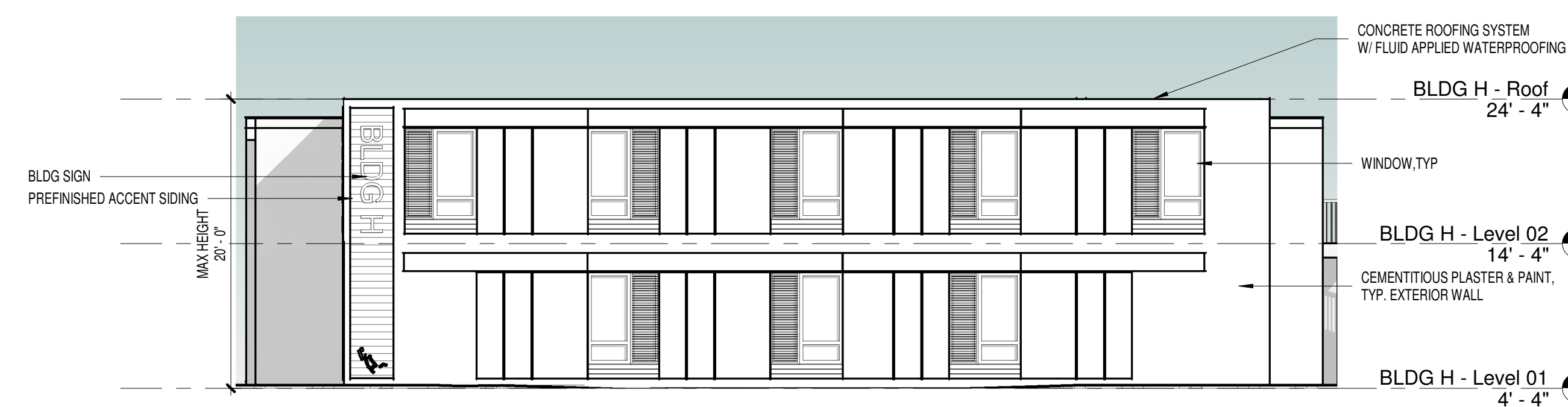
2 BLDG H - NORTH ELEVATION A-H2.0 SCALE: 1/8" = 1'-0"
