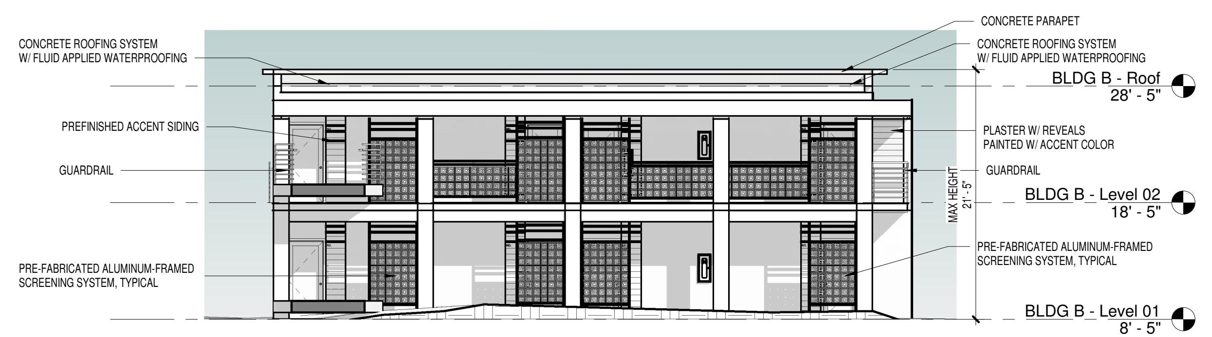
2 BLDG B - WEST ELEVATION A-B2.0 SCALE: 1/8" = 1'-0"
