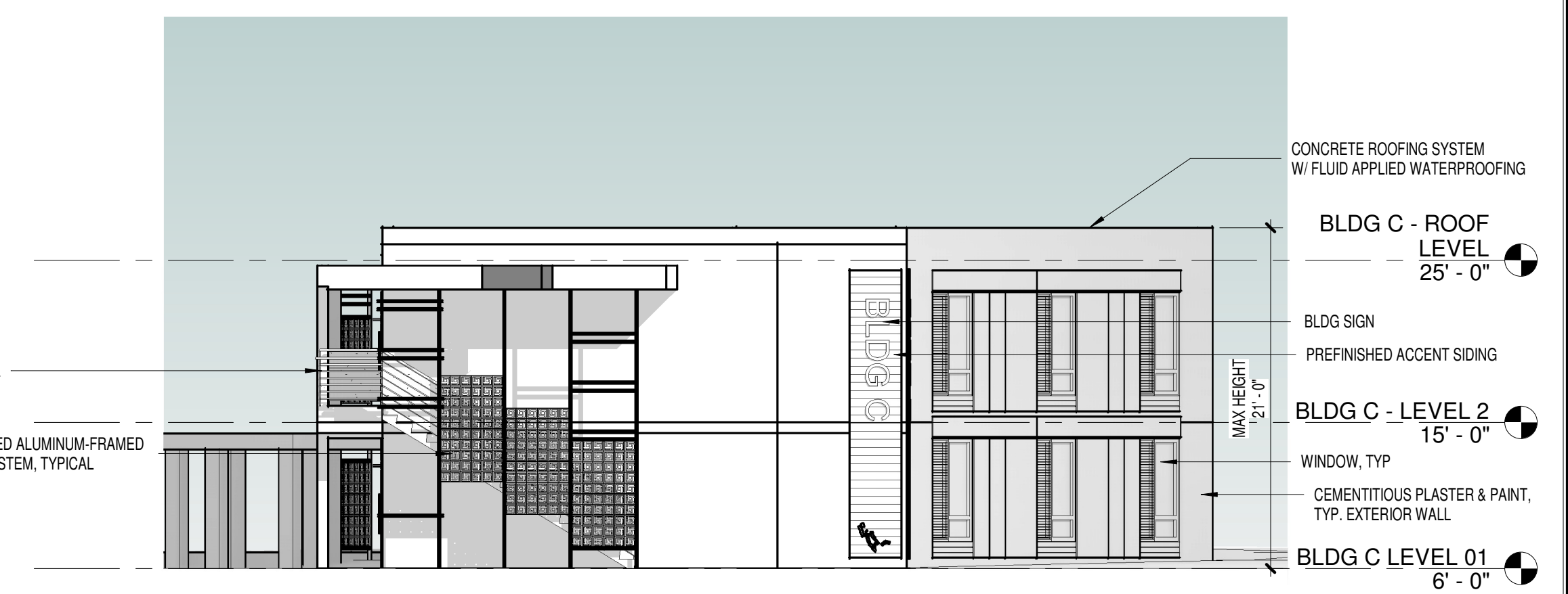
3 BLDG C - EAST ELEVATION A-C2.0 SCALE: 1/8" = 1'-0"
