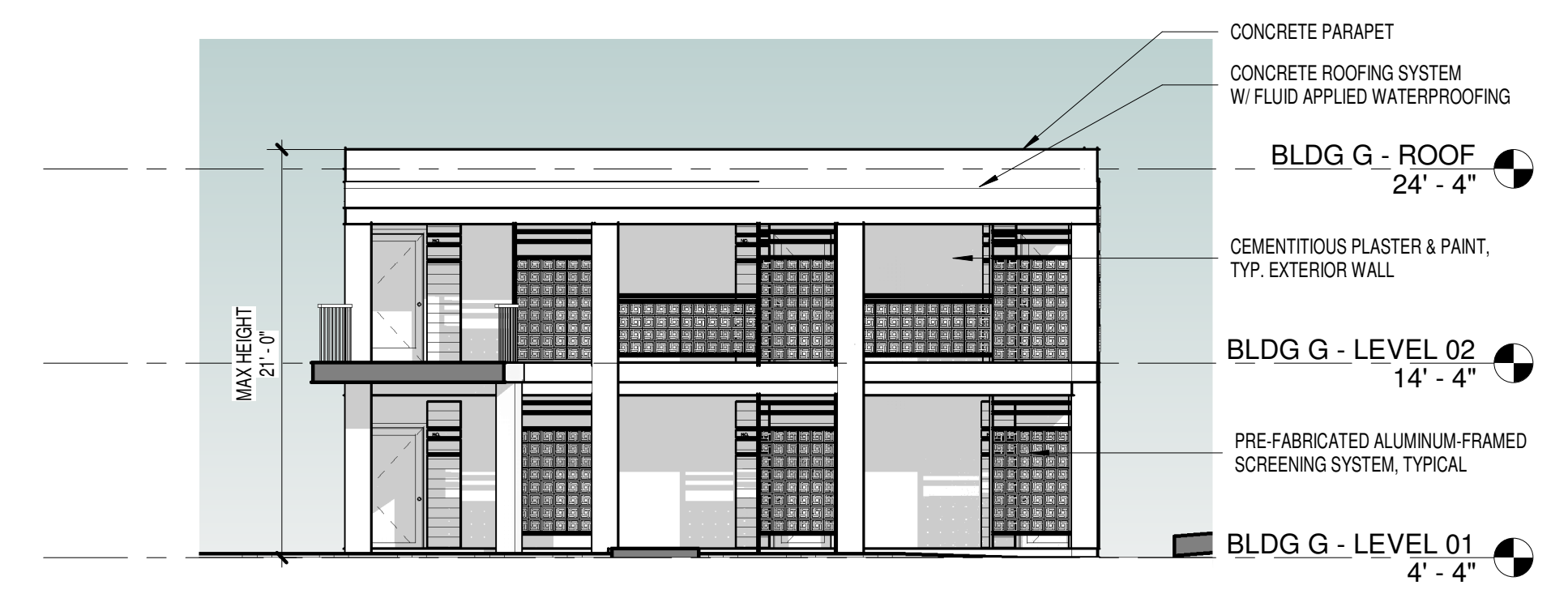
2 BLDG G - SOUTH ELEVATION A-G2.0 SCALE: 1/8" = 1'-0"
