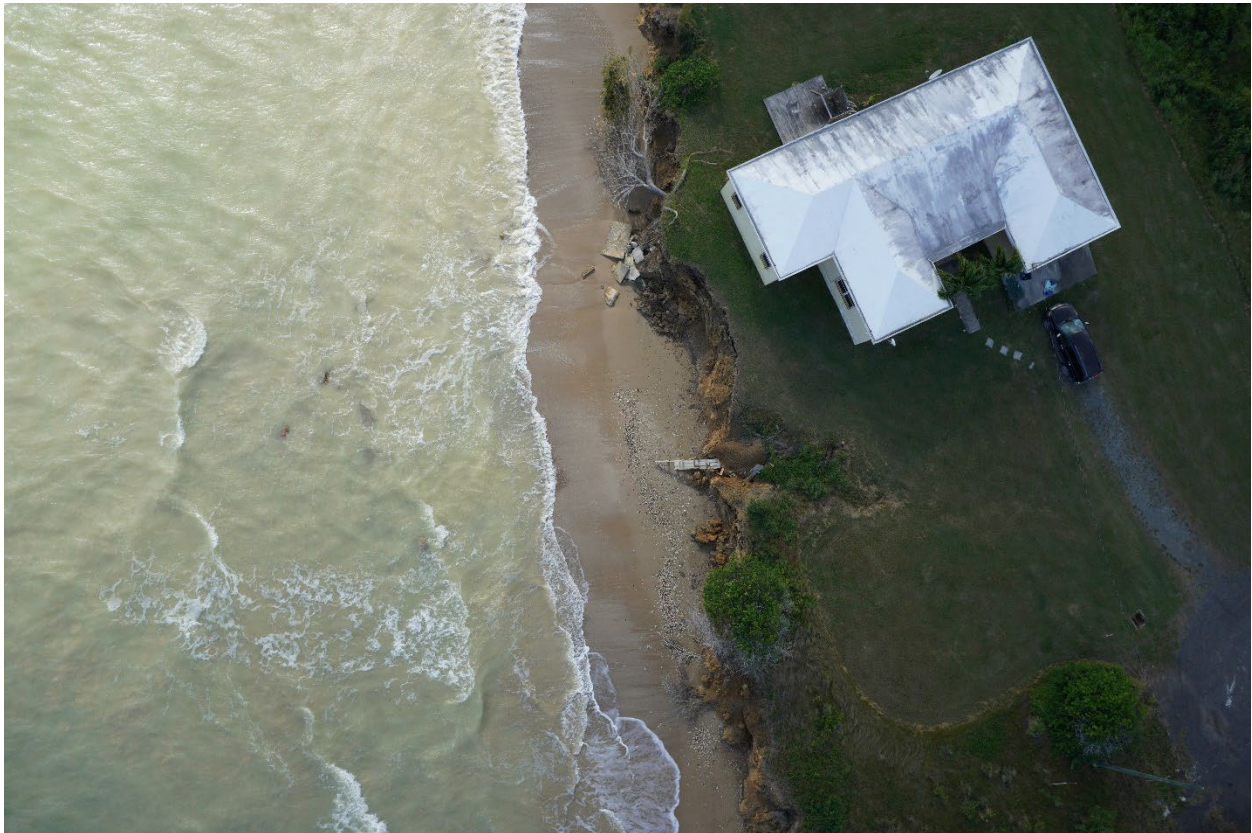
Figure 44. Coastal erosion due to sea level rise threatens stability of homes near the coast (note photo is from another area on St. Thomas and not within the Dorothea watershed).
