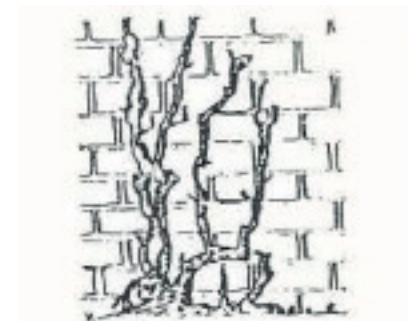
Subterranean termite trails - frequently a sign of termite presence.
