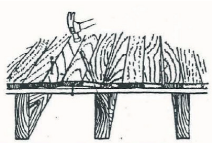
Warped or lifting decking can often be repaired. Always try to repair existing materials rather than replacing wholesale.
