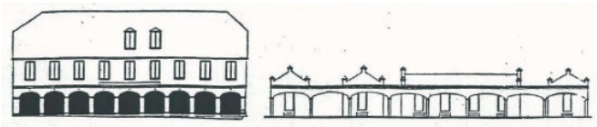
More recent arcades often fail to duplicate essential features of historic examples. The modern arcade in the right hand picture - built of reinforced concrete - allows too great a span for arches, which in turn rest on columns too small (visually) to support them.
