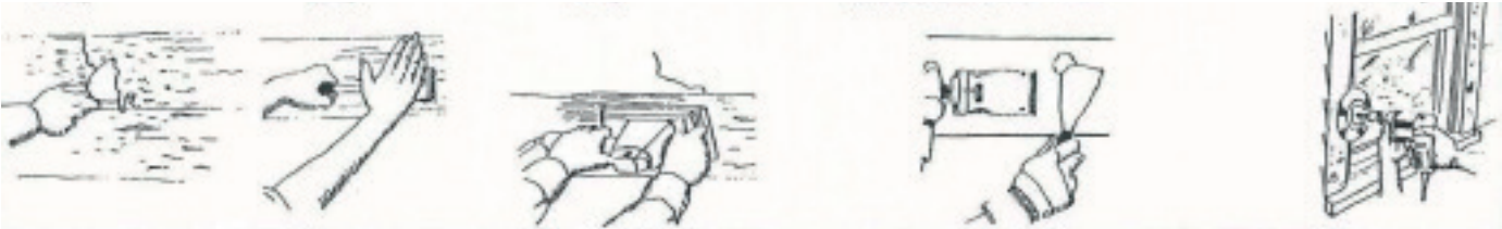
For paint preparation use (1) a putty knife (sometimes combined with chemical strippers); (2) a paint scraper; (3) an orbital sander; and (4) a heat plate (with caution). Do not use disk or belt sanders, both of which can mar wood surfaces.
